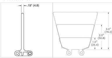
**Flights**Standard flights are available in 1", 2", and 3" heights. Standard flight indent is 1" or greater from outside edge of belt
