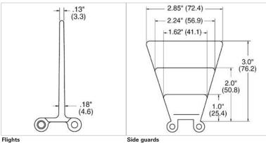
Standard flights are available in 1", 2", and 3" heights. Standard flight indent is 1" or greater from outside edge of belt
